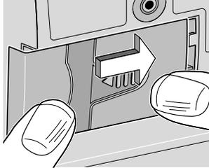
5. Ensure that the door is latched by trying to remove the door without pressing the arrow button.
