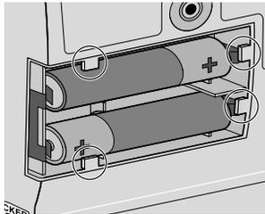
In order to install or replace the batteries, be sure the pump is **Stopped**. Then, follow these steps:
