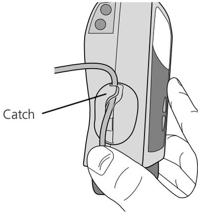
3. To seat the tubing into the groove, gently pull the tubing upward, until it is under the retention nubs and flat in the groove.
