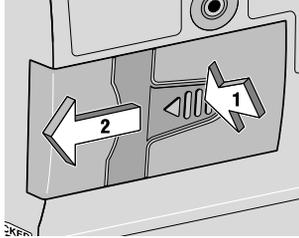
2. Remove the used batteries. Pulling on the end of the battery strap will make battery removal easier.
