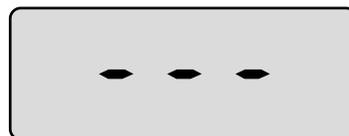
**STEP 2:** After the third dash appears, release the STOP/START key. The word “STOP” will flash on the display. In this example, the display shows a RES VOL value of 28 ml.
